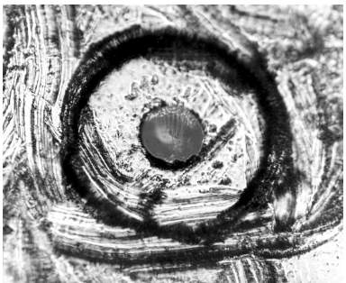
Figure 1-14. Damage from improper cleaning.
